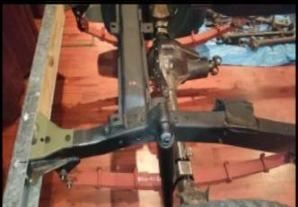
Work has commenced on paint removal from differential using a wire wheel in preparation for new painting.
