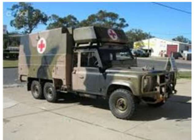
Ambulance body, 6x6, air conditioned, power steering, turbocharged diesel
