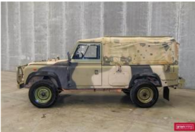
Perentie 110, Fitted For Radio (FFR) fitted with separate 24 volt electrical system, provision for carrying 4 extra 12 volt batteries.
