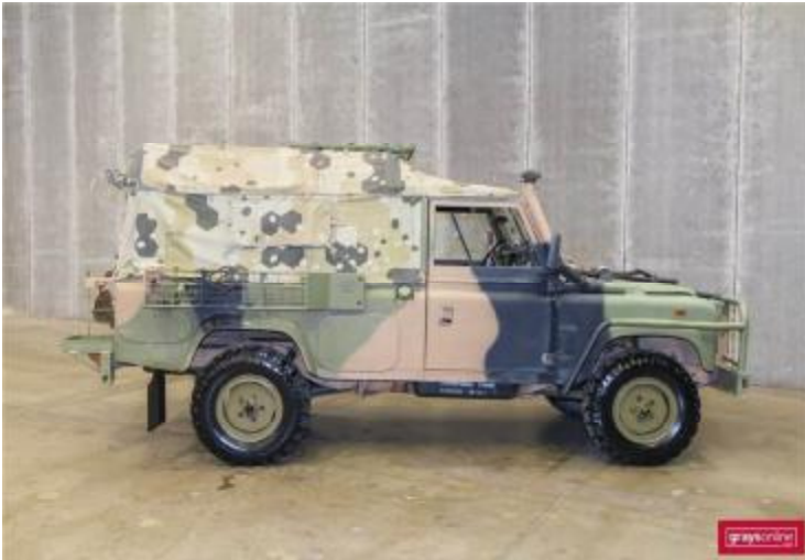
Perentie 110 4x4 Regional Force Surveillance Vehicle (RFSV) Fitted with PTO winch, power steering, twin fuel tanks, raised air intake.
