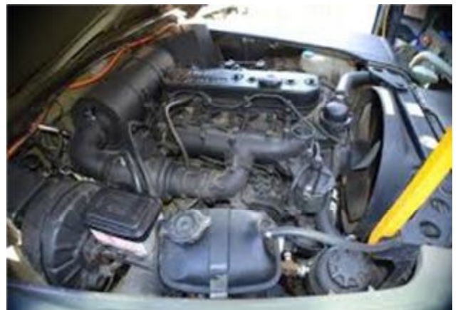
Isuzu 1BD1 diesel engine 4 cyl, 1.8 liter, direct injection. Bore : 102 mm, Stroke : 118 mm, weight approx. 350 kg. Power 78 kw, torque 263 Nm.
