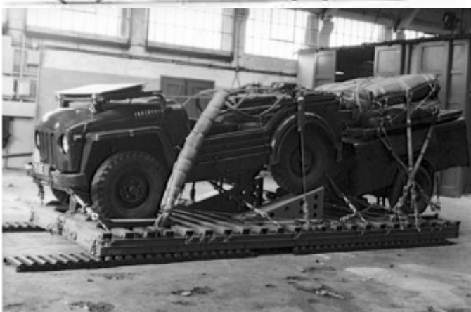
The Champ during Air drop trials. This proved unsuccessful, with the Champ being too heavy (around twice as heavy as the WW2 Jeep)
