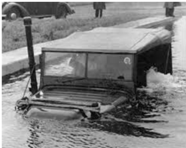
The wading trough can be filled to a depth of four feet, is mainly used by prototype military vehicles.
