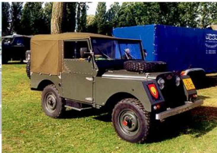
↑ The Minerva, built under license from Land Rover, by the Belgian car builder of the same name. In 1952, Land Rover won the contract for 2500 vehicles, which were supplied in CKD form, to be assembled by Minerva. Chassis, axles, transmission, and other parts were supplied, but the contract specified 63% of the parts should be of Belgian origin. The body was made of steel. The front mudguards were squared off and sloping, which were easier to produce. Just under 10,000 of these vehicles were produced, and supplied to the Belgian Army and Police.
