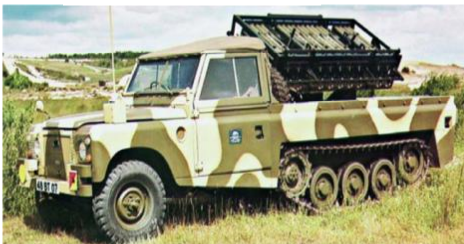
↑ The Minerva, built under license from Land Rover, by the Belgian car builder of the same name. In 1952, Land Rover won the contract for 2500 vehicles, which were supplied in CKD form, to be assembled by Minerva. Chassis, axles, transmission, and other parts were supplied, but the contract specified 63% of the parts should be of Belgian origin. The body was made of steel. The front mudguards were squared off and sloping, which were easier to produce. Just under 10,000 of these vehicles were produced, and supplied to the Belgian Army and Police.
