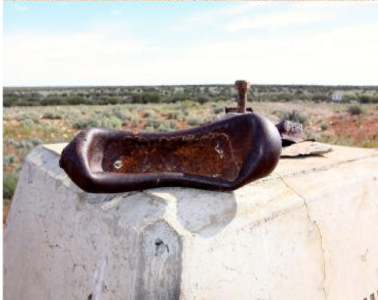
Pictured above is an old steel oxygen bottle, recovered from one of the test sites. The force of the blast caused it to implode ! It was made of ¼" thick steel !!
