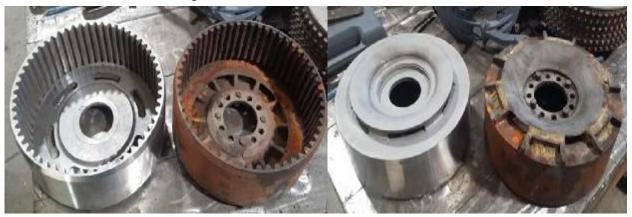
I have assembled the steering clutches but not the fine adjustment yet. I guess that will be done after installation as I don't have details of that part so a bit of trial and error to come. I have just temporarily put the newly made clutch cover on for a bit of a test fit and it is excellent.
