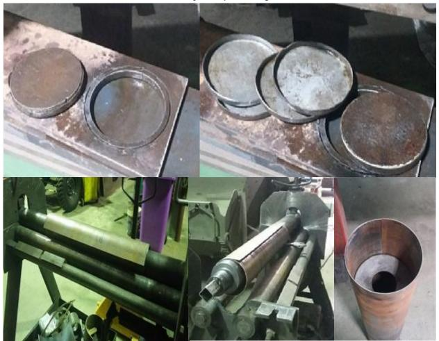
I made a really crude press die and formed the ends as per the drawing I have and some baffles for the inside. Rolled the tube to suit the ends and welded it all together. Also the clamping brackets as well.
