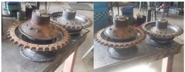
I had to complete the rest of the turning clutch drum. The chap that cut it for me left excess so I can do my welding and then machine it down to size.
