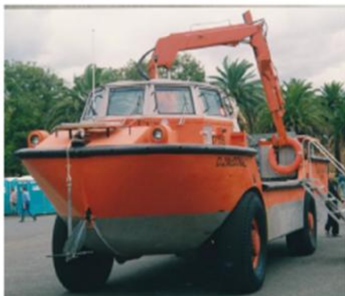
A LARC V of the ANARE Detachment on display at Victoria Barracks, Sydney 1994. This vehicle has the later orange hull top, and the HIAB crane is mounted. (P. Handel photo)
